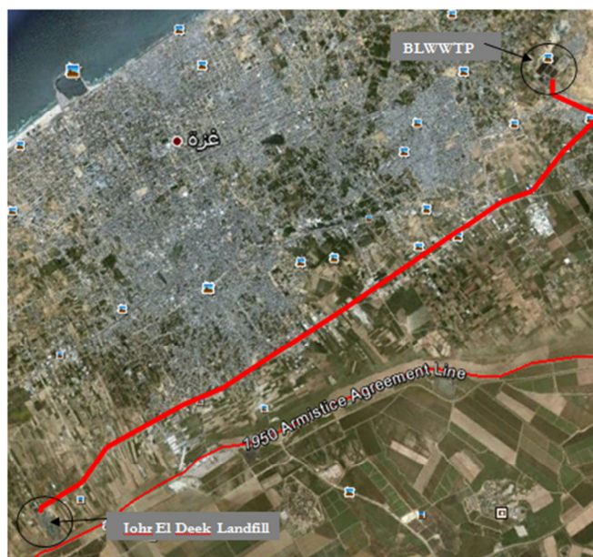
Figure 5.15 Proposed Route to Transport the Soil from Jehr Eldeek Landfill to Effluent Lake Adjacent to BLWWTP (if needed)
