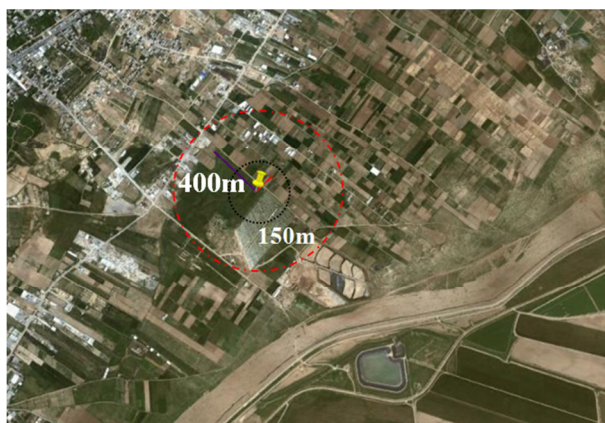
Figure 5.3 Buffer zones (150 m radius) around the main noise sources during construction of water distribution network (booster pump and storage tanks)
